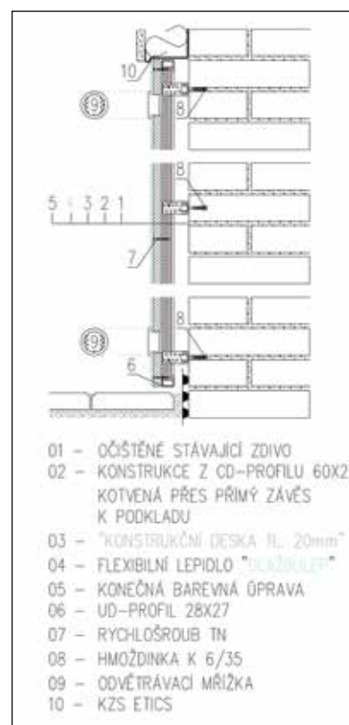
Obr. 5 - Sanace soklu KD
